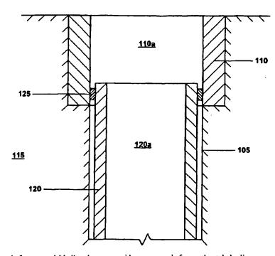
(57) Abstract: The end of an expandable liner hanger provides a receptacle for another tubular liner.
